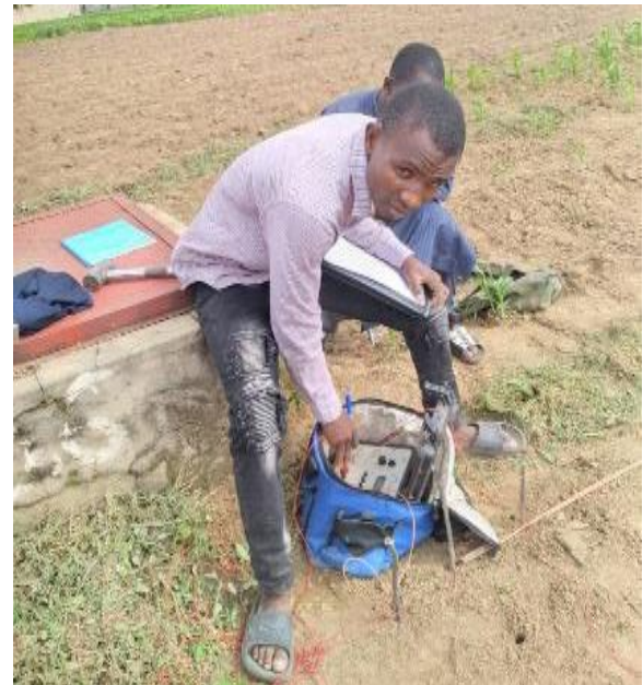
Figure 6: A pictorial presentation on carrying out resistivity survey using Hummel method conducted beside the existing borehole (0.5 meter).
