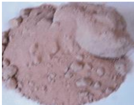
Figure 1: Numan Natural clay bonded silica sand
