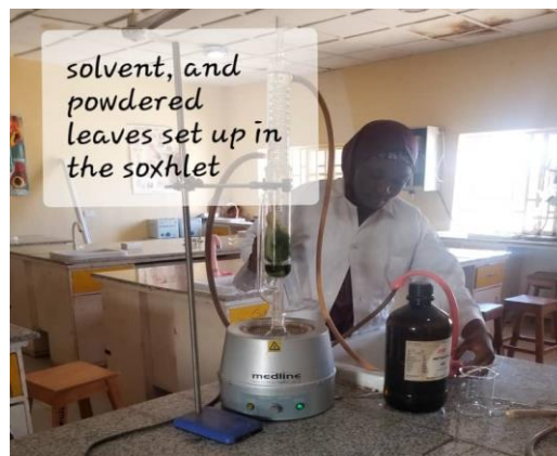
Figure 4: Soxhlet extraction unit being set up
