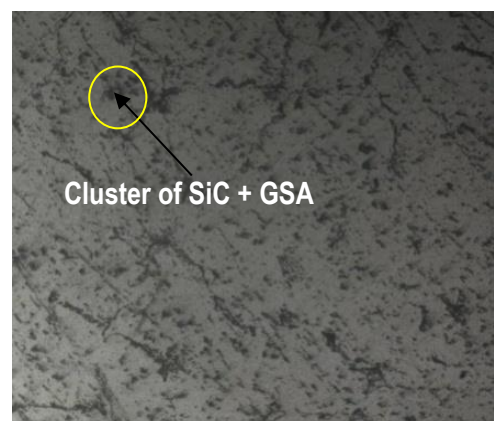
Figure 5(d). Microstructure of composites 12g SiC+GSA reinforcement
