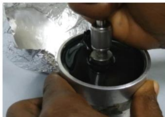
Figure 2: Bitumen testing by Coaxial probe
