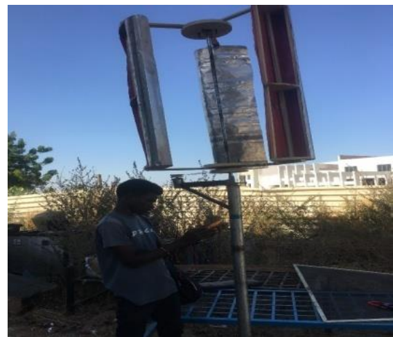
Plate1.The Micro-Vertical Axis Wind Turbine Physical Model on Test
